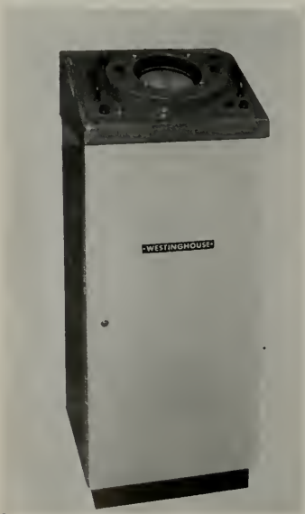
Closeup of continuous plan position indicator scope for Westinghouse Marine Radar set. This type of scope, with the ship in the center, provides a continuous picture of ship traffic and shoreline conditions throughout a range of from 100 yards to 32 miles of the vessel.
